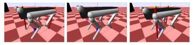
Fig. 2. HyQ trotting in place in simulation. The left and right images show the robot in two consecutive mid-stance phases. The middle image shows the robot in flight phase. The red cylinders represent ground reaction forces.
