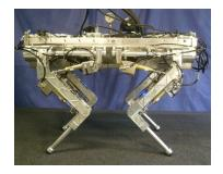
Fig. 1. The hydraulically actuated quadruped robot - HyQ. It has 12 degrees of freedom and its size is comparable to a goat. HyQ is designed for highly dynamic behaviour, e.g. trotting and jumping (http://youtu.be/wPxXwYGZmd8).
