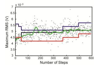
**Figure 2** Preliminary data of soleus muscle activity of the contralateral limb during the first experiment (contralateral limb controls the level of assistance provided to the ipsilateral limb). The trial lasted 10 minutes. *Dots*, maximum RMS per step; *black line*, average RMS over constant condition; *green line*, filtered moving average of RMS over 10 steps; *red line*, lower threshold; *blue line*, upper threshold.
