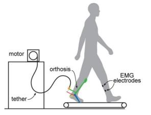
**Figure 1** Depiction of experimental setup 1. An able-bodied subject walks on a treadmill with the AFO worn on the right leg. The AFO is attached to an off-board motor via a flexible tether. EMG electrodes on the contralateral limb measure soleus muscle activity for control of the assistance provided to the ipsilateral limb.
