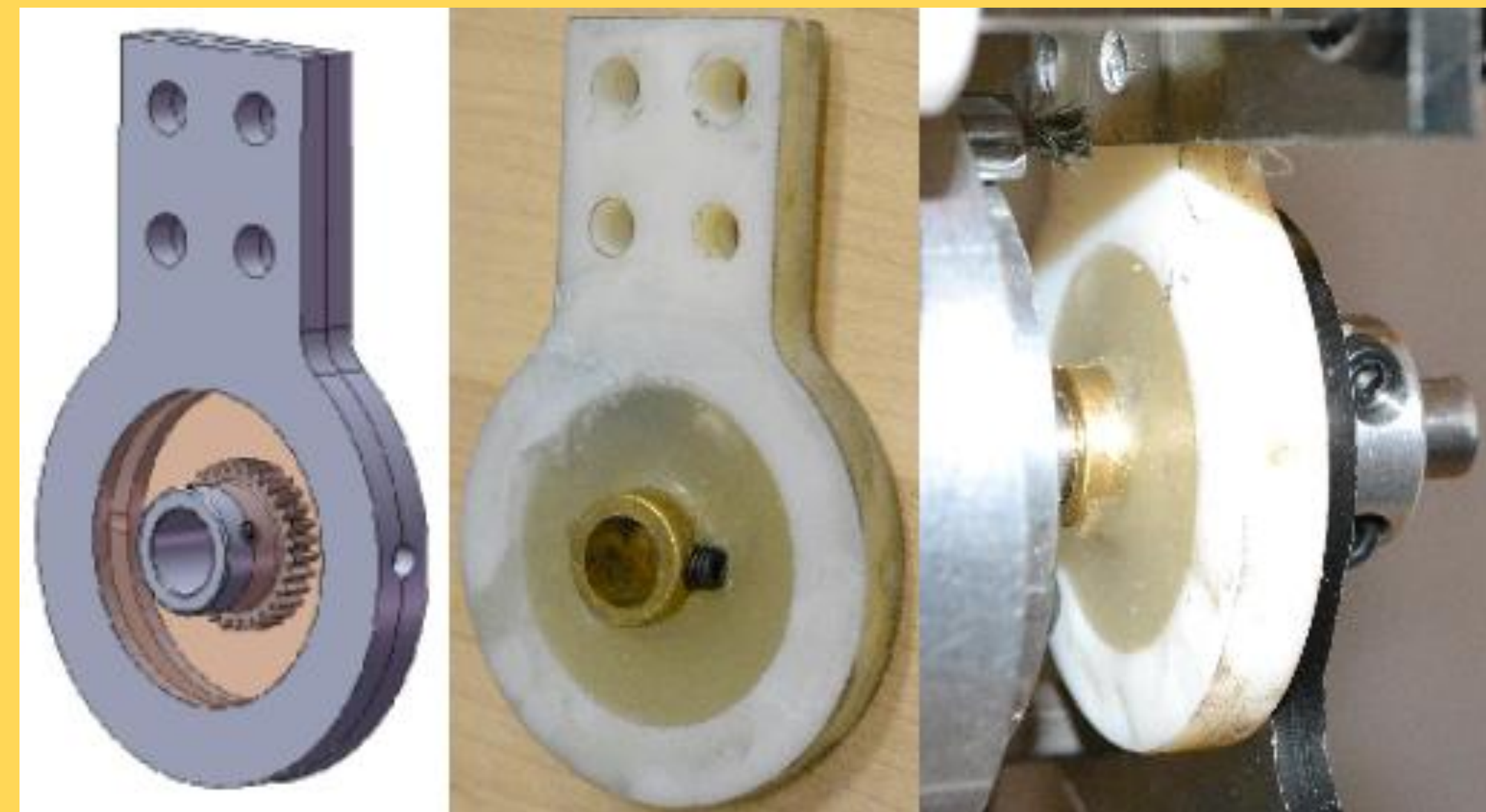
Fig. 3: Floating compliant joint. (L) Concept. (C) Prototype. (R) Implementation.
