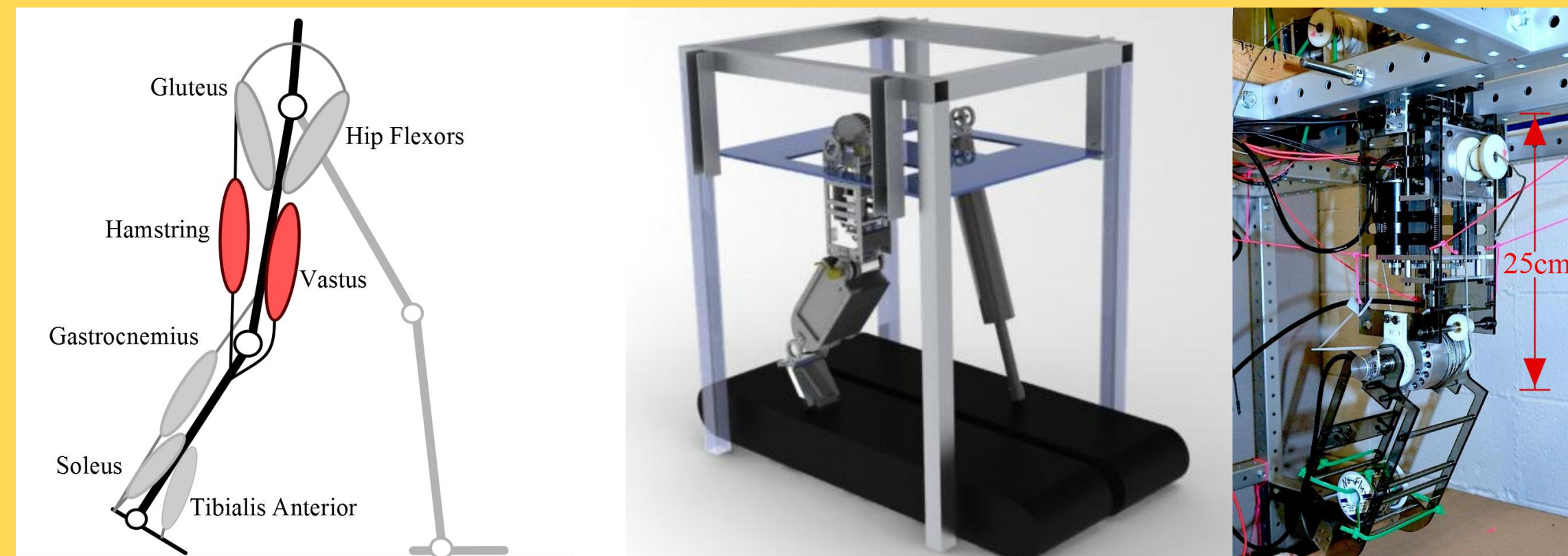
Fig. 1: Robotic testbed development. (L) Major human leg muscles with monoarticular knee extensor and biarticular knee flexor highlighted. (C) Testbed concept. (R) Current robotic implementation of RNL. Thigh coupled to cage for experiments.
