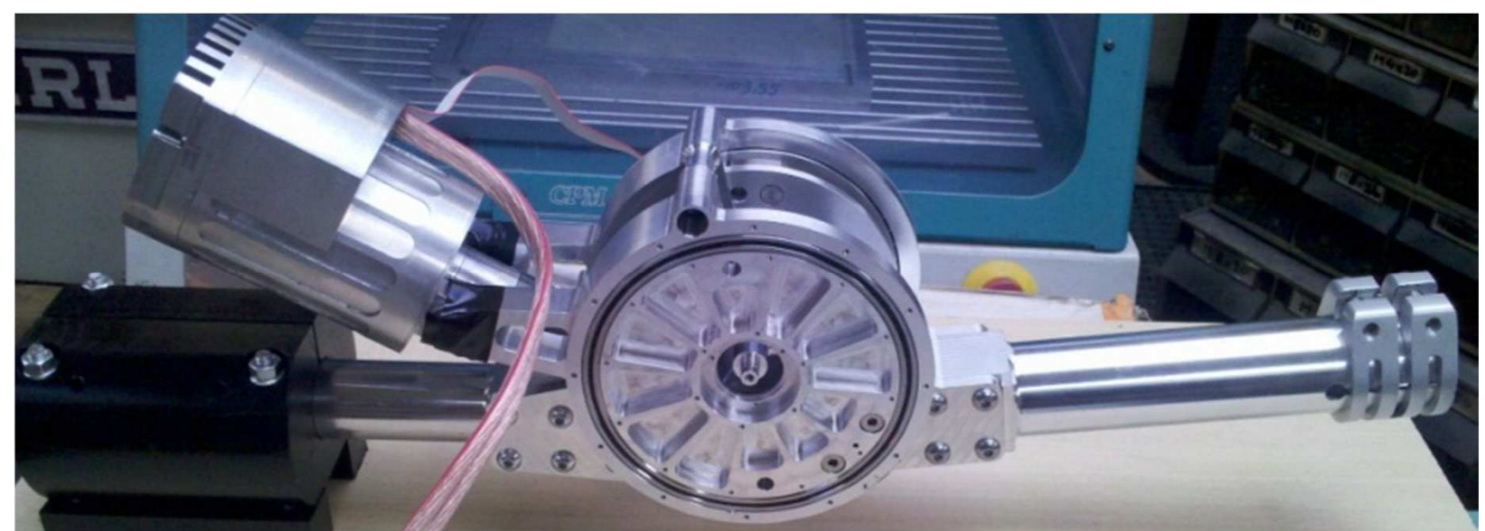
Fig.2 Exoskeleton knee joint: the joint (excluding the segment tubes) weighs 2.9kg; electronics responsible for low-level control and EtherCAT communication are contained inside the center of the joint; motor drive electronics are embedded inside the actuator.
